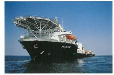
MSV "MAXITA" is designed for most types of offshore work, including subsea installations, heavy lifts, laying of flexible flowlines, umbilicals, cables and small rigid steel lines, burying of subsea lines etc. All types of offshore construction work which requires a very good DP capability.
